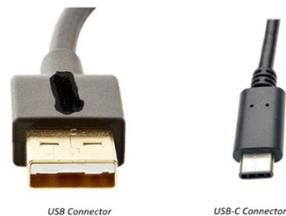
What the connector can do electrically is defined by the protocol. The old protocols are USB and USB-2. These are used for mice, thumb drives, and other simple devices. Besides data, the port can provide 5 volts to power the device.
