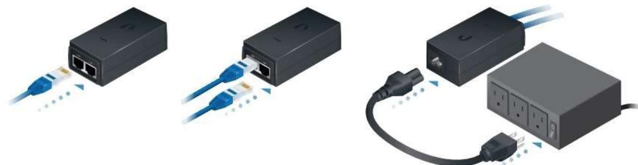
*Figure 2 Power Injector*
